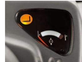
The interlock state is also indicated on the meter panel.
