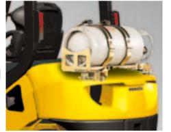
**The sunken counterweight\* specification truck with an expanded rear view area.**
