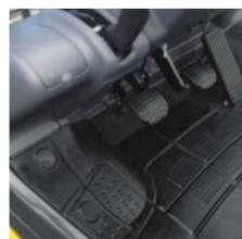
The wide, flat floor accommodates the tilt cylinder under the floor. Suspended (type) pedals are used to provide extra foot space, which significantly reduces operator fatigue. The new wide-open, non-slip step and spoon-curved fender makes getting in and out easy and safe.
